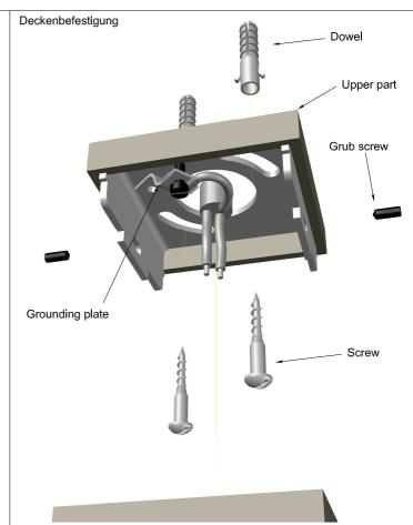
Place the upper part on the mounting plate and fasten it to the ceiling with screws and dowels.
