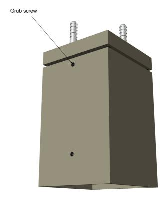
Place the luminaire on the mounting plate and screw in the grub screw. CAUTION! Please only screw in flush with the luminaire housing. Do not screw in too far.
