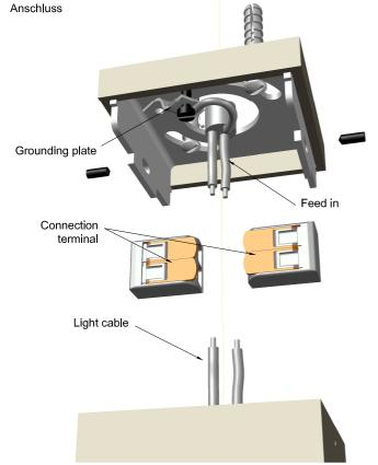
Connect the ground conductor of the supply cable to the grounding plate and connect the supply cable to the luminaire cable using the enclosed connection terminals.
